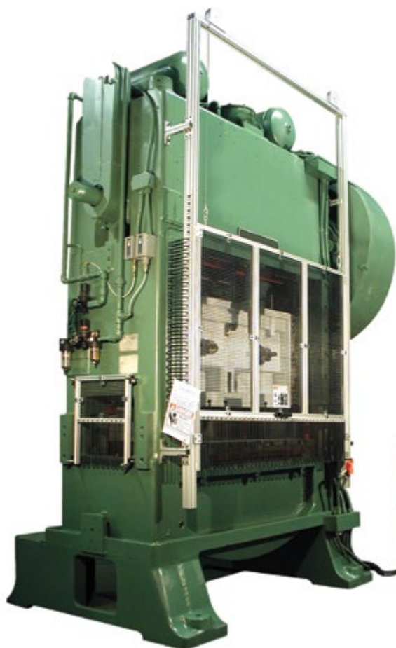
Spring-Lift Guard on a Straight-Side Press With Adjustable Side Guards
