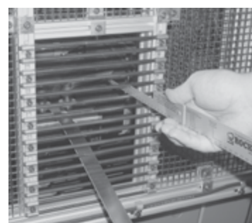
Guard-opening scale being used to check openings for compliance
