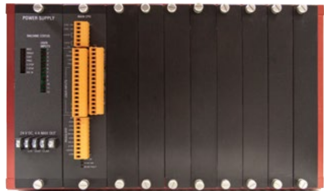
Main Control Rack With Power Supply and Main CPU Card
