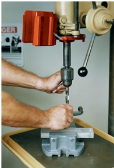
Front hinge shield shown open for tool change.
