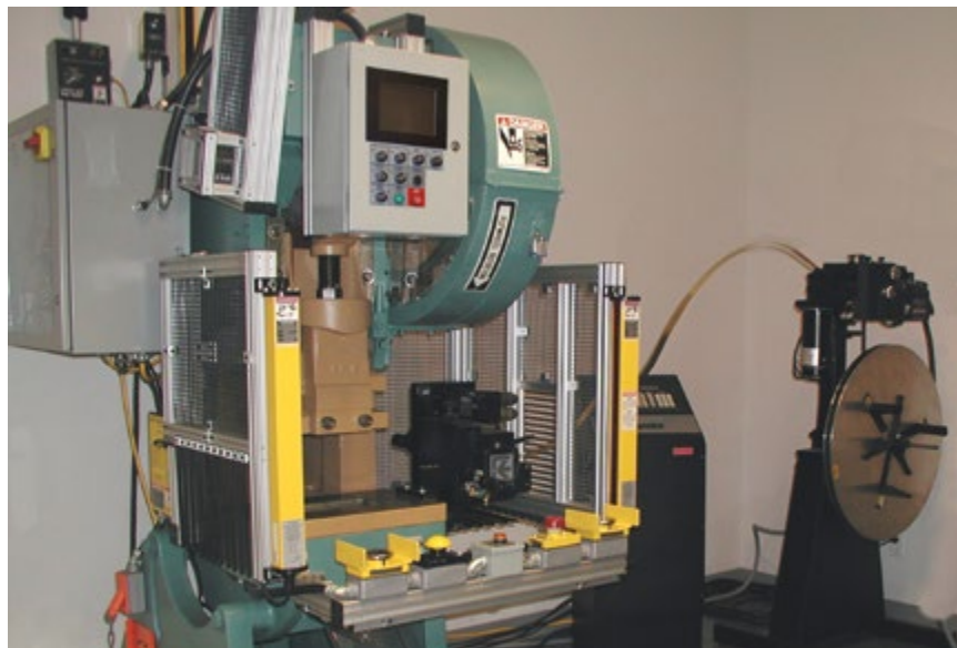
OB1 With Press Automation System and Servo Feed Interface
