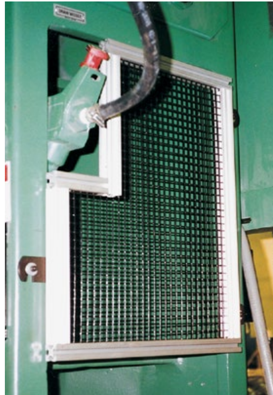
Single-Panel Barrier Guard With Notched Upper Left Corner Mounted on Back of a Machine
