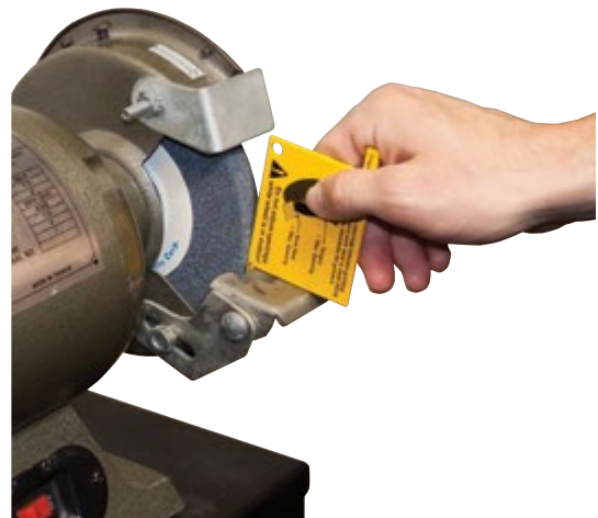
Checking work rest opening.
