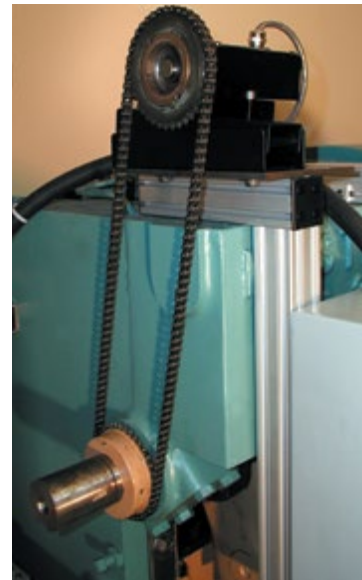
Resolver/Pulser Assembly on Press (Sprocket and chain cover has been removed for photo)
