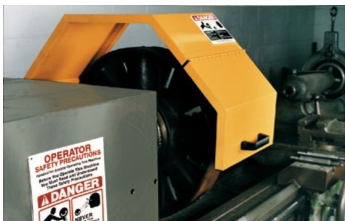
The hinged portion can swing up for workpiece changes.
