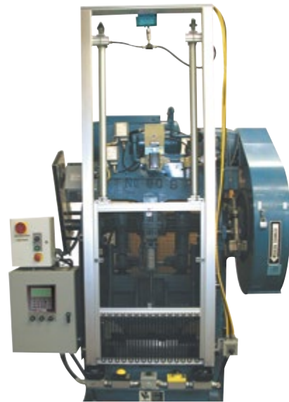
Point-of-Operation Light Curtains on a Press
