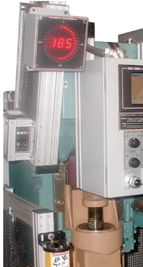
Crankshaft Angle Display Mounted on a Mechanical Power Press
