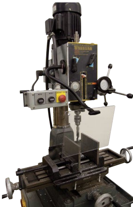
Flexible spring-steel arm shield on milling machine.
