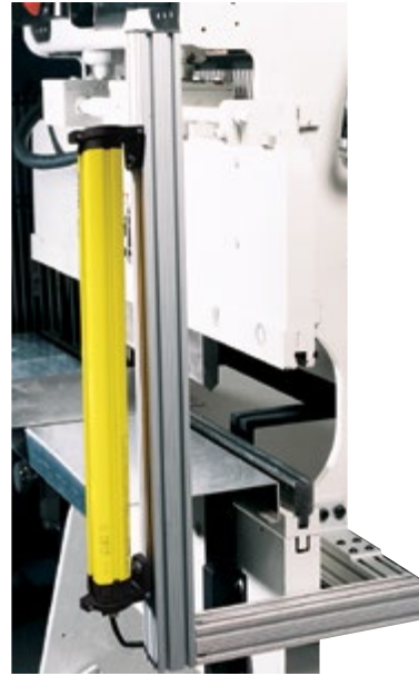
3-Section (OBI) Stationary Light Curtain Mounting Bracket (barrier guard has been removed from machine for photo)
