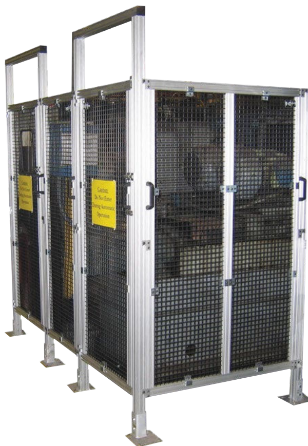
Perimeter Guard Around a Transfer Line
